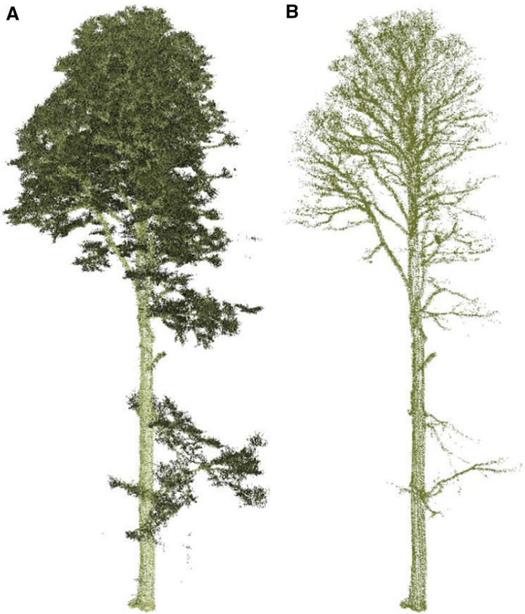
Fig. 5 A single European beech ( F. sylvatica ) in the high-density point cloud acquired by the Brown Platform for Autonomous Remote Sensing. a All returns. b Only returns with 16-bit reflectance intensity > 45,000. The intensity filter removes leaf material and shows branch and stem structure necessary for automated segmentation
