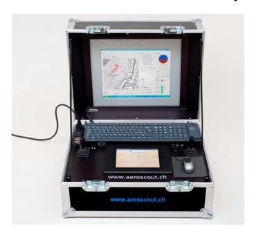
**GENERAL** The Aeroscout Advanced Ground Control Station (AGCS) with its touch screen provides all capabilities in order to operate the Aeroscout unmanned autonomous helicopter systems, in particular the Scout B1-100 UAV helicopter. This includes mission planning, mission control, display of UAV status information, and UAV performance monitoring.
