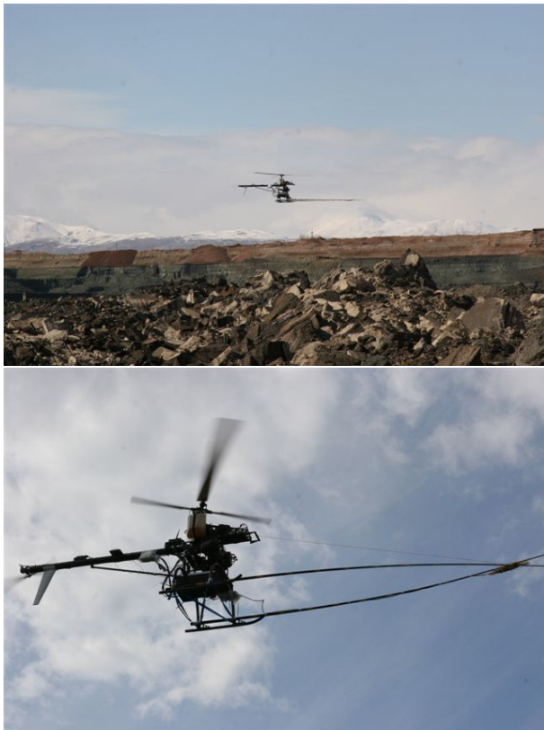
Figure 9: Applied automatic mission flight for aerial magnetic sensing at the coal mining site mentioned above.
