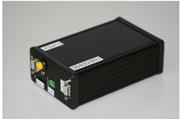
Figure 3: Picture of the magnetic data acquisition module developed at Lucerne University for Applied Sciences and Arts.
